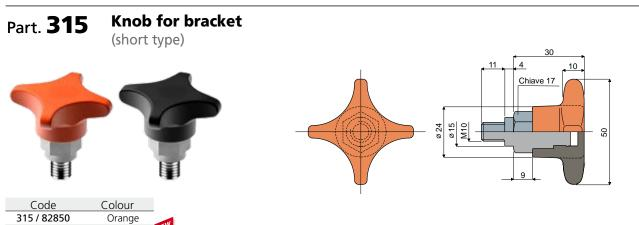
MATERIALS: Knob made of reinforced polyamide orange or black colour; threaded bushing made of nickel plated brass. FEATURES: Accessory to be used with head Part.223. BOX QUANTITY: 24 pieces.
