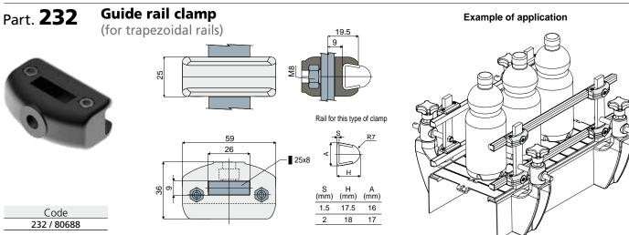
MATERIALS: Clamp made of reinforced polyamide black colour; bolts and nuts made of stainless steel AISI 304.
