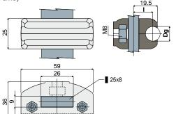
MATERIALS: Clamp made of reinforced polyamide black colour; bolts and nuts made of stainless steel AISI 304.
