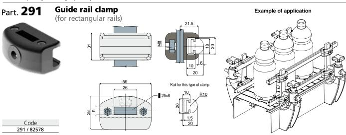
MATERIALS: Clamp made of reinforced polyamide black colour; bolts and nuts made of stainless steel AISI 304. FEATURES: Supplied assembled. To be used with flat profile with sizes 25x8 mm. To be used for the support of the product guide rail Part.373. BOX QUANTITY: 24 pieces.
