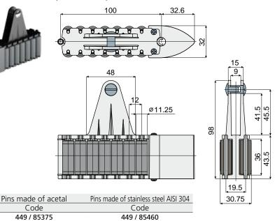
MATERIALS: Rollers in polyethylene grey colour; module in acetal resin black colour; shoe in acetal resin grey colour; support pins in black acetal or in stainless steel AISI 304.
