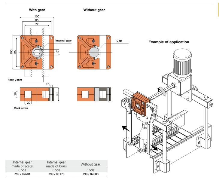
MATERIALS: External body of reducer is made of reinforced polyamide orange colour; self-threading screws are made of stainless steel AISI 304. Available: without internal gear; with internal gear made of acetal, white colour; with internal gear made of brass.
