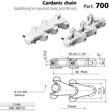
MATERIALS: Chain made of natural acetal; notch made of polyamide; pin made of stainless steel AISI 430.
