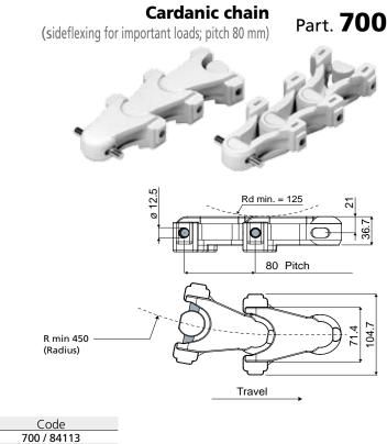
MATERIALS: Chain made of natural acetal; notch made of polyamide; pin made of stainless steel AISI 430. FEATURES: To be used in the conveyor systems; for important loads (breaking load: 19600 N). BOX QUANTITY: 3,040 meters.
