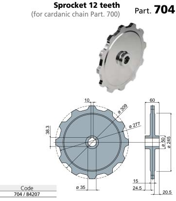
MATERIALS: Sprockets in zinc plated steel. FEATURES: To be used with chain Part.700. BOX QUANTITY: 2 pieces. ON REQUEST:
